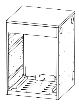
Attach the left + right side panels to the inside with 3 truss head screws each.
