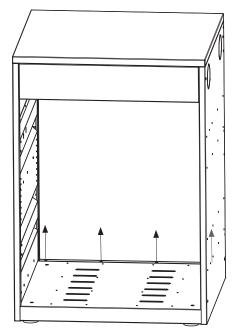
Attach the base plate to the back panel with 4 truss head screws.
