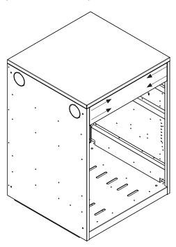
Attach the top reinforcement panel with 4 M4 1b stainless steel nuts for Dekton countertops.
